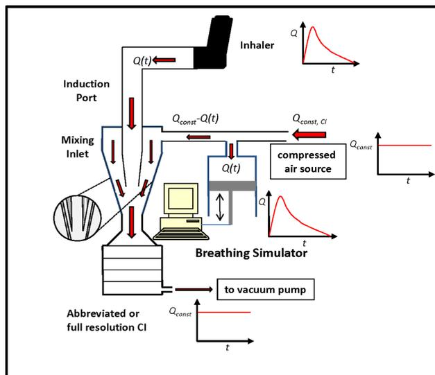
Figure 2: Miller Inlet (Nephele Enterprises, through RDD Online, Virginia Biotechnology Research Park, VA, USA and Copley Scientific Ltd., UK) Enabling CI Operating at Constant Flow Rate ( $Q_{const}$ ) to Interface with Breathing Simulator Providing Variable Flow Rate ( $Q$ ) for pMDI Testing
