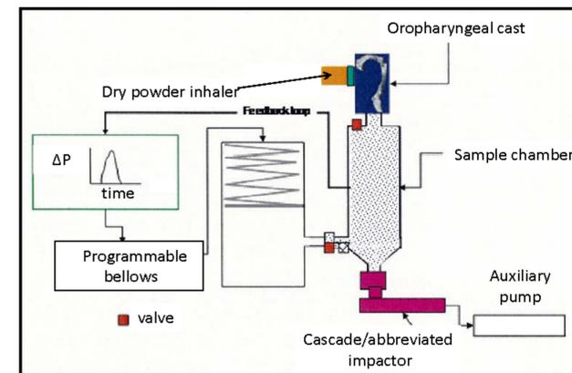
Figure 3: Electronic Lung™ Used in the Testing of DPIs with Actual Patient Inhalation Flow Rate–Time Profiles (from Good Cascade Impactor Practices, AIM and EDA for Orally Inhaled Products, Springer, April 2013)
