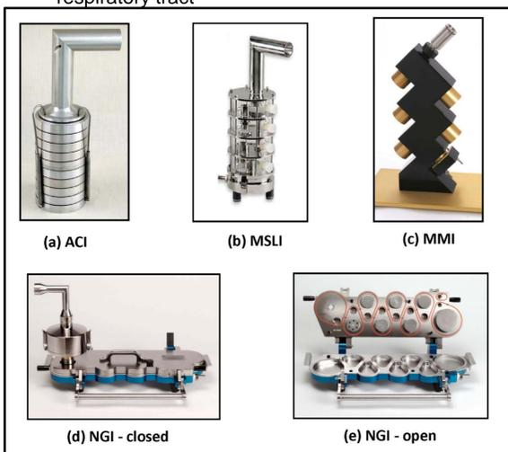
Figure 1: Widely Used Cascade Impactors
